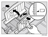
**3** Lift the paper delivery end plate and move it to match the print paper size.
